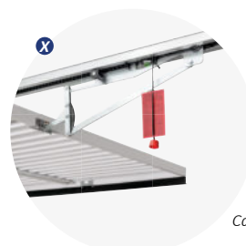
Typical Up-and-Over Garage Door with Canopy Gear
